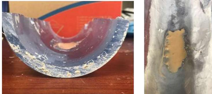
Figure 7. Experimental setup of settled kaolin in a mock PVC pipe cut in half to simulate gravity-drained conditions.
