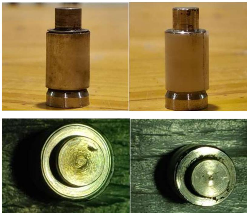
**Figure 94. Eroded Coupon surfaces removed from the elbow and bottom sections of the pipe.**
