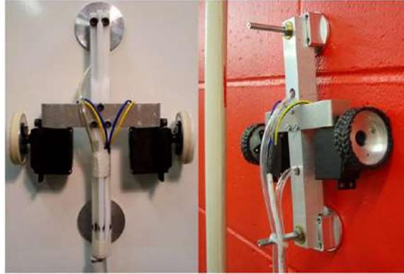
**Figure 61. NCAP robot equipped with non-contact grippers [21].**
