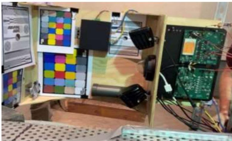
**Figure 83. Cameras and sensor system electronic component set up board for radiation chamber testing SWRI [20].**
