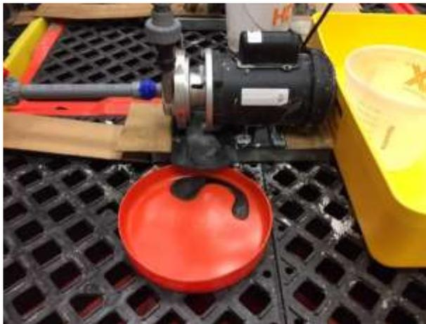
**Figure 113. Pump leaking from seal.**
