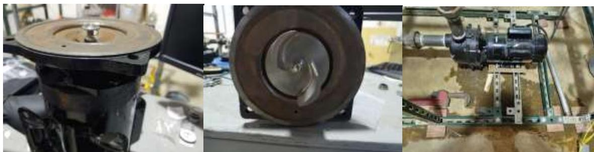
**Figure 86. a) Pump assembly stages (left and center) and b) assembled pump - leakage after testing (right).**
