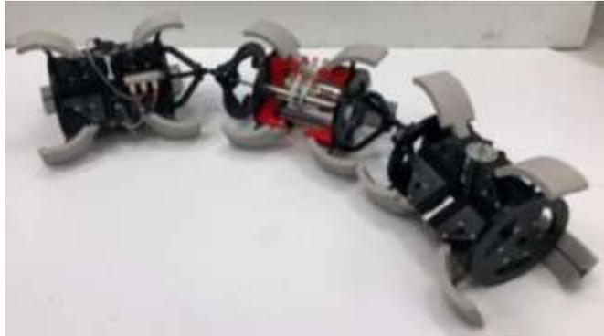
**Figure 32. Mother pipe crawler prototype.**
