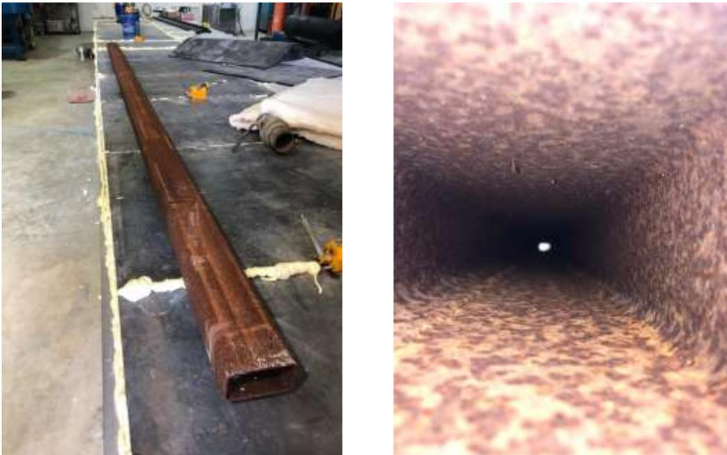
Figure 20. Corroded surface setup.
