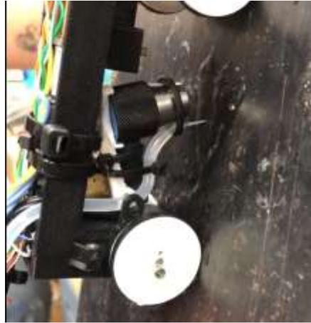
**Figure 24. Water pumped as a couplant.**
