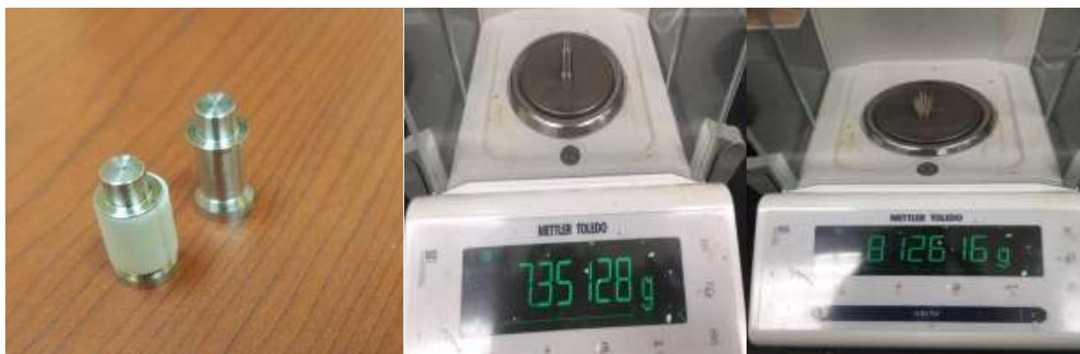
**Figure 84. a) SRNL coupon b) coupon weight (without sleeve) and c) with sleeve.**
