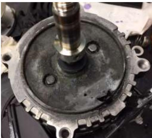
**Figure 116. Motor face with eroded hole.**
