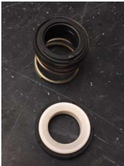
**Figure 117. Mechanical seal from pump #2.**
