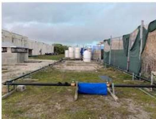
**Figure 2. Pipeline constructed for flushing experiments.**
