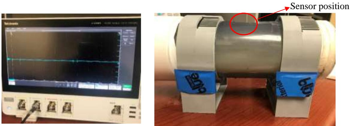
**Figure 5. (Left) Tektronix MSO44 Mixed-Signal Oscilloscope (Right) Experimental Setup of settled kaolin in a mock 3-inch PVC pipe for fully-flooded conditions.**
