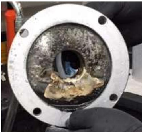
**Figure 114. Pump #2 backplate showing leakage from mechanical seal location (Seal removed).**
