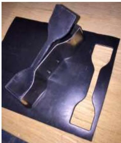
**Figure 108. Dog bone cut from a sheet of EPDM.**
