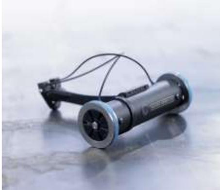
**Figure 67. ReconRobotics Recon Scout magnetic ship climber [38].**
