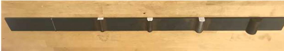
Figure 19. Half-round weld seams with different heights.
